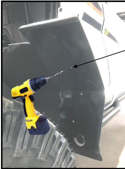
Fender flare guides holes (7x)
