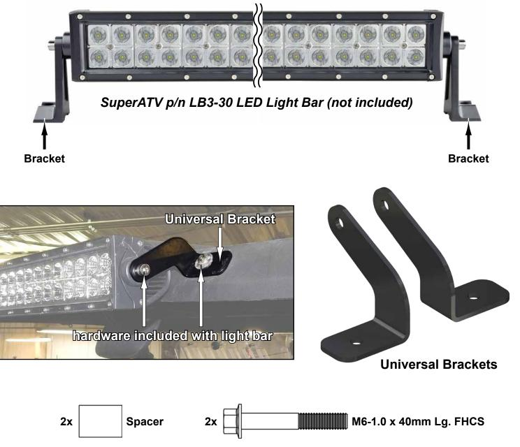
(Use when installing 40" LED Light Bar onto Polaris General<sup>™)</sup>
