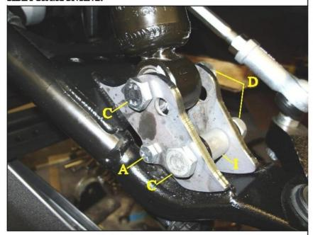
PLACE THE PLATES ON THE FRONT SIDE OF THE STOCK MOUNTING TABS. INSERT THE SPACER AND TIGHTEN TO FACTORY SPECS.
