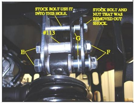
THIS IS A TWO POSITION LIFT THE PIC U SEE IS SET TO THE HIGHEST POSITION WHICH WOULD BE APPROX. 3". IF YOU ONLY WANT 2" USE THE HOLES ON RIGHT OF PLATES.
