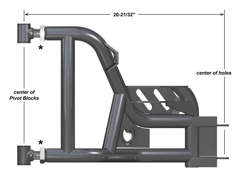
\*Leave Jam Nuts loose. Tighten after final adjustments have been made.
